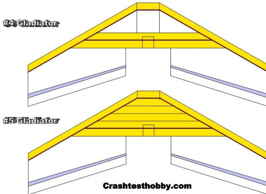
**3. Image #4 shows the Reinforced Tape pattern for the top of the wing. We recommend "Scotch Extreme Tape"**
