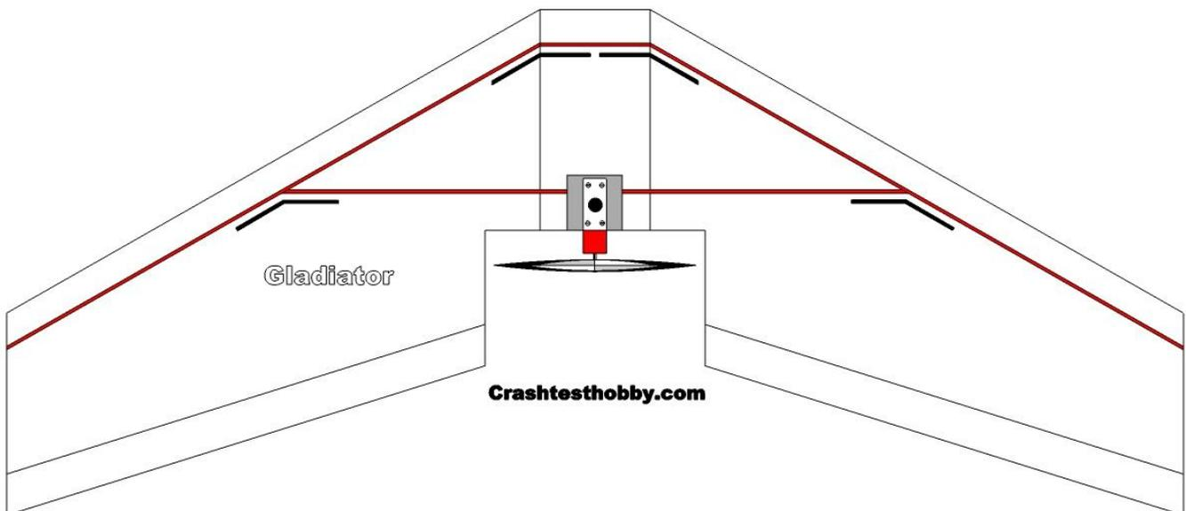
The spar location on the top and bottom Gladiator are the same. The fiberglass spars are installed directly over each other to create an "I beam" type structure that is many times stiffer than one spar alone.
