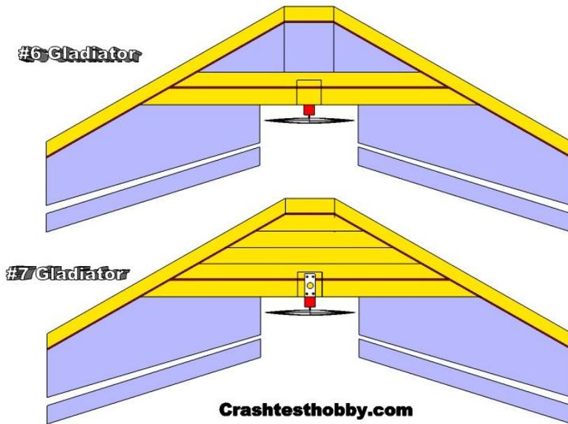
**5. Images #6 and #7 show bottom and top details of the laminated wing and the mounting of the motor.**
