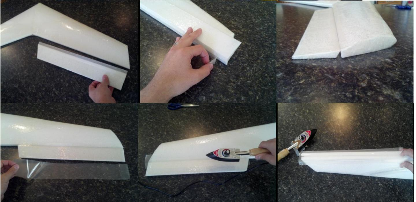
7. Image #7 shows the tape hinges and suggested radio installation.
