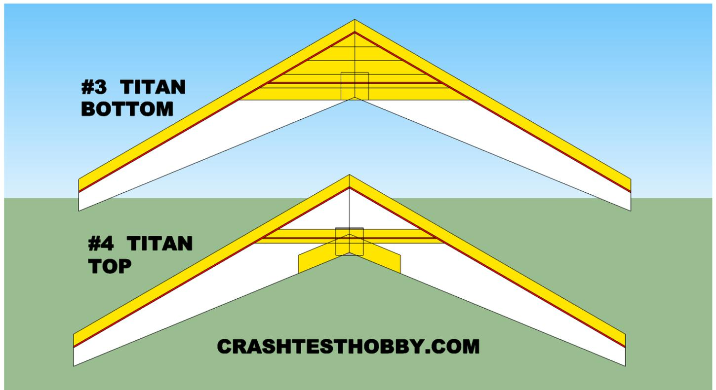
**3. Image #3 shows the Reinforced Tape pattern for the bottom of the wing. We recommend "Scotch Extreme Tape"**
