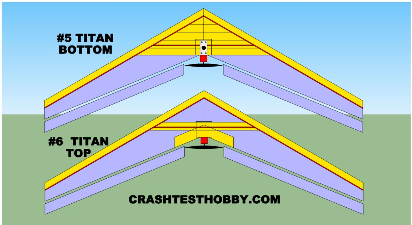
**5. Images #5 and #6 show bottom and top details of the laminated wing and the mounting of the motor.**
