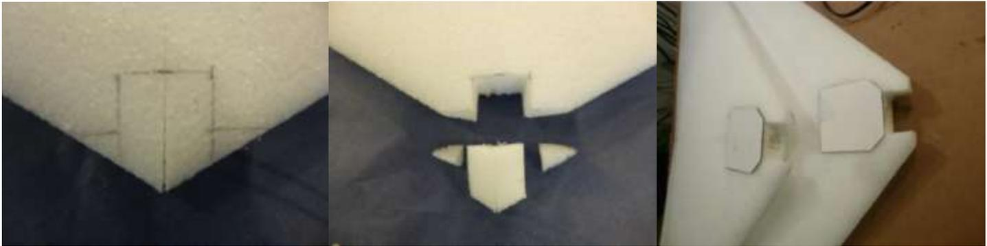
10. Before cutting the motor cutout, measure and mark the CG of the plane. The 36" Roswell CG is back 7.25" and the CG on the 29" Roswell is back 9" from the nose of the plane. Put a mark on the bottom of the plane to be used later with radio installation.
