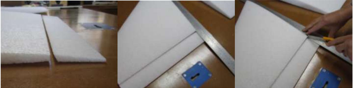
3. Cut your elevons to length. The inside edge of the elevon will be in a straight line with the inside edge of the wing section. If you are building the 29' Roswell-2, the inside edge of the elevon will be at an angle to the inside edge of the wing section.
