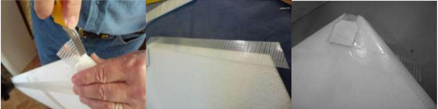
**UV PROTECTED CLEAR LAMINATE** - is Included in the kits. It protects the foam from moisture and dirt and adds a lot of strength. It protects the Extreme Tape that is sensitive to UV light.
