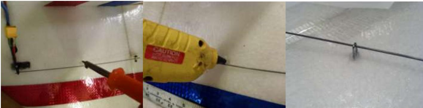
75. Remove the servo arms, slide the push rod through the hole in the servo arm, and place the end of the push rod through the EZ Connector, then set the servo arm back on the servo. You may have to drill the servo arm for the rod to fit.
