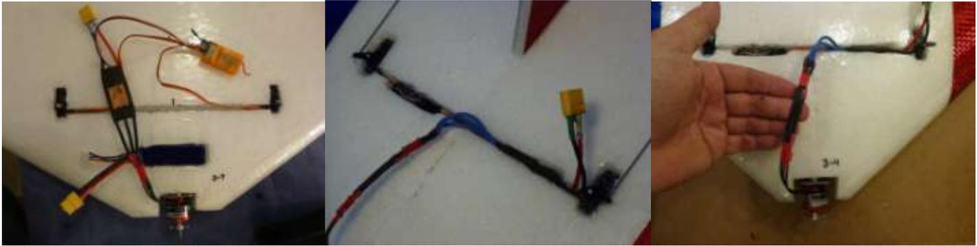
59. All of the wires are tucked in the slot except the battery wire to the ESC and the ESC to motor wire connection.
