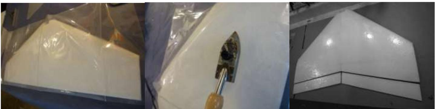
**COVERING EPP ELEVONS** – Cover the elevons with two layers of laminate to make them stiff (comparable to balsa wood).
