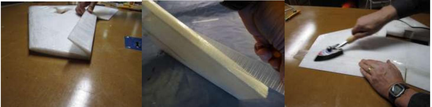
48. Cut 2" (5cm)-wide strips of laminate the length of the elevon. Cover the 1" (2.5cm) strips of tape you just placed, top and bottom, and iron the laminate in place. Make sure, as you iron, that the elevons end up flat and flush with the wing, not bending up in places. If they seem to be pulled in places, reheat the area with the iron, and lay an object over the elevon to keep it flat as the laminate resets.
