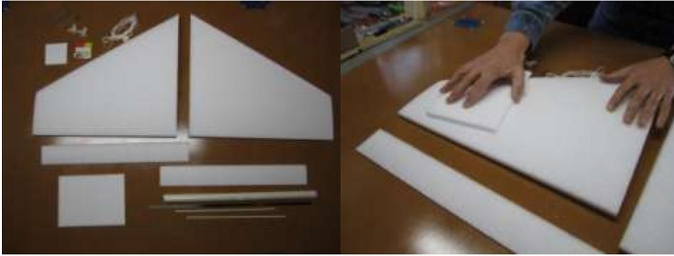
**The 36" Roswell has a straight trailing edge. The 29" Roswell-2 is swept.** The 29" wing is faster and more aerobatic but the narrow wing experiences more prop torque on take off until it is up to speed. This means it needs a faster launch.
