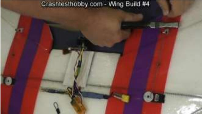
Cut slits for velcro strap to hold battery in place.
