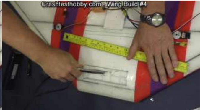
Cut a slot for the ESC and receiver.
