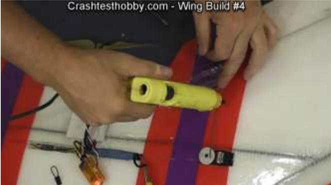
Wire guide should be tight enough to keep pushrod from flexing.
