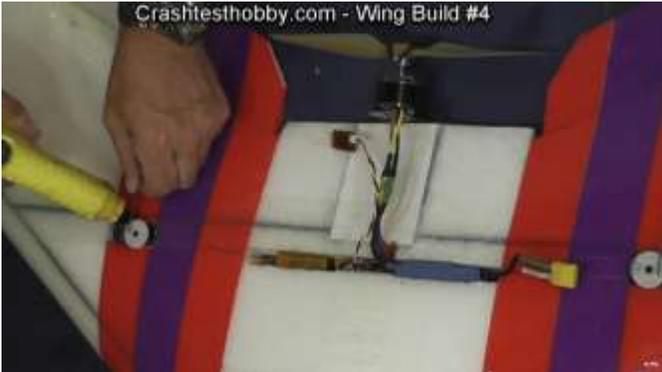
Punch hole for staple to make pushrod wire guide.
