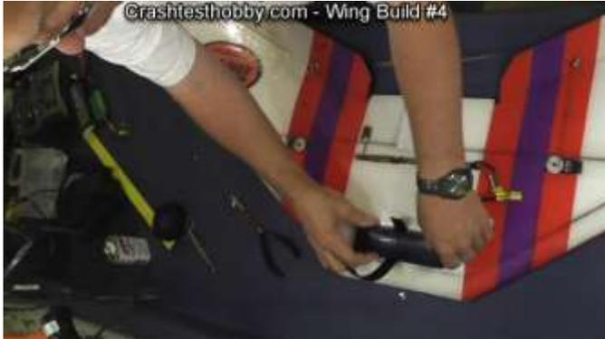
Fit ESC into slot. Enlarge hole for air flow to cool ESC.
