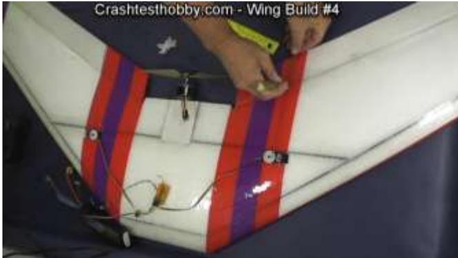
Enlarge hole slightly with soldering iron for glue.
