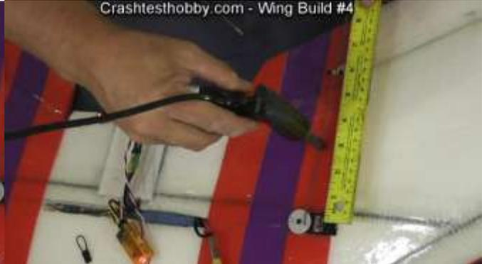
Put glue in hole and press staple into place.
