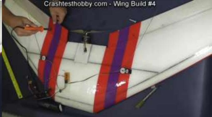
Glue horns in place working glue up through slit.
