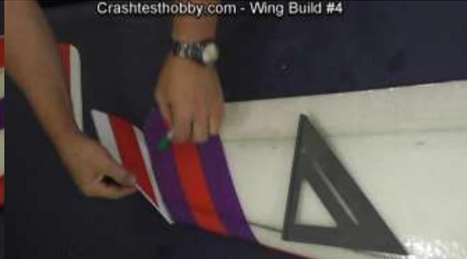
Use soldering iron or razor blade to cut 1" slit.
