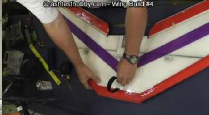
Place battery in place and secure with the Velcro.
