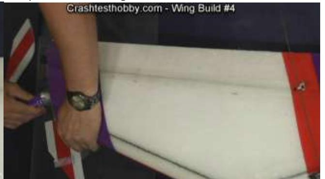
Tape fin in place and allow glue to dry.
