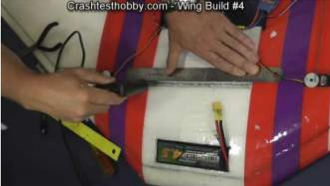
Cut slits and push the servo wires into the foam.
