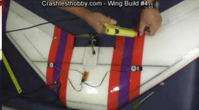
Drill out TOP hole in horn for EZ connector with 1/16th bit.
