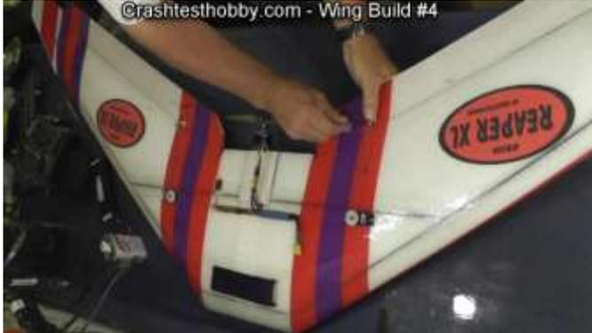
Angle of bottom of elevon should be angle of bottom of wing.
