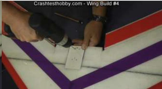
Screw the motor mount in place.
