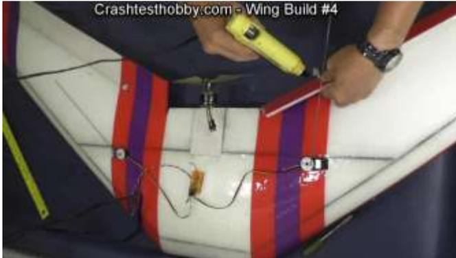
Apply glue on the top of the wing to secure horn.
