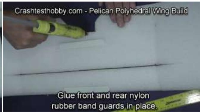
Using a medium temperature hot glue gun glue on the nylon reinforcing braces to protect the foam from being torn by the rubber bands. This is the end of the stock wing build.
