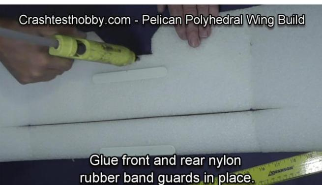
Using a medium temperature hot glue gun glue on the nylon reinforcing braces to protect the foam from being torn by the rubber bands. This is the end of the stock wing build.
