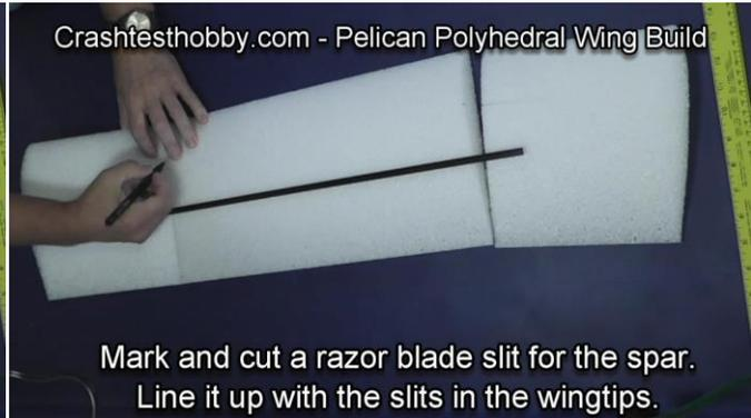
The center spar will go through the slits in the wingtips on the poly wing. Mark the central spar location by lining up the tips with the main wing core. Lightly sand the carbon spar. Use a metal straight edge and a new razor blade and cut a 1/2" deep slit across the top of the middle core of the wing. Press the carbon fiber spar into place with the spar centered with the same amount of spar poking out of each side.
