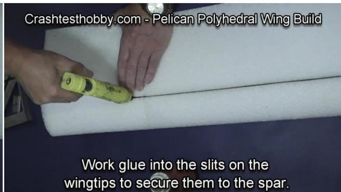
Using the hot glue gun work several pumps of hot glue in the spar slit in the wingtip to secure the spar from both the top and the bottom. Make sure the wingtip is still 3.5" off the table while the glue cools.
