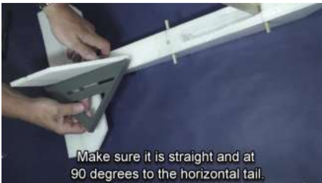
Punch some holes through the laminate and glue the vertical stabilizer in place.
