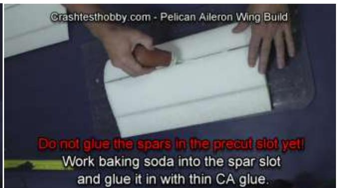
Put baking soda along the spar and work it into the slit with the carbon spar. The baking soda acts as a catalyst and speeds up and hardens the CA glue. Glue the spar in to the slit with thin CA glue.
