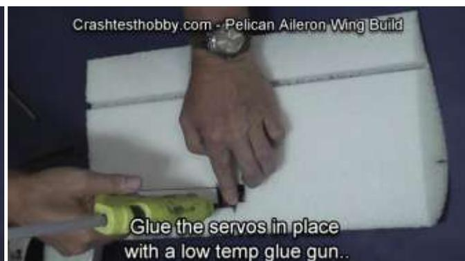
Before gluing the servos in place with a low temperature glue gun, bind them to the radio and center the servo arms on the servo. Drill out the third hole in the servo with a 1/16" bit to be big enough for the push rod. Don't glue the servo extension wires in except for where they exit the wing in the middle where they will be plugged into a Y connector that plugs in the receiver.
