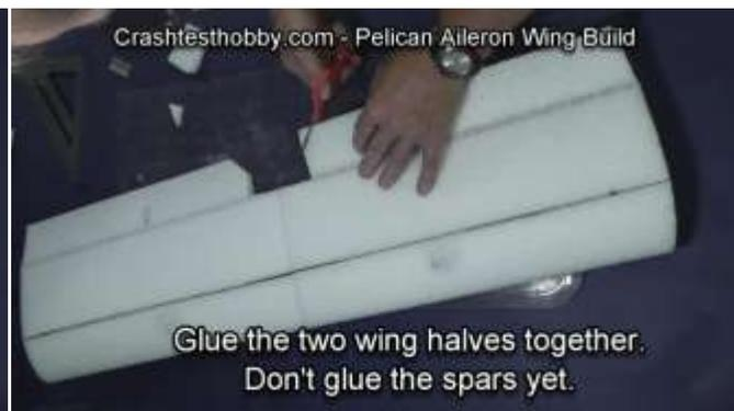
**Glue the wing halves together. Apply glue to the center spars after you have the wing positioned with the tip 3.5" off the table. Squeeze liberal amounts of glue in to support the spars where they cross in the middle of the wing.**
