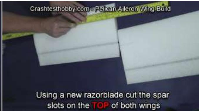
Cut a spar slit, with a new razor blade, on the top of the wing for the flat carbon spar. This slit should be the same distance back as the precut slot already in the wing. Lightly sand the spar to help the glue to stick. Press the spar into the slit with the extra spar at the center of the wing.
