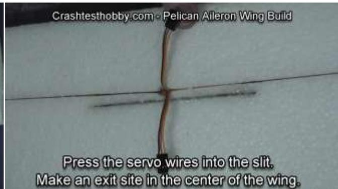
Make a hole at the exit point for the servo wires to exit the wing. Glue the nylon protectors on the front and back of the wing with a low temperature glue gun to prevent the rubber bands from tearing the wing.
