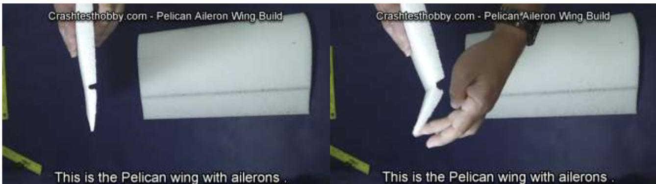
The ailerons are already precut into the wing core. Fold up the ailerons and flex the wing to loosen up the hinges.
