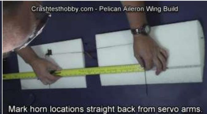
Install the control horn in straight behind the servo arm with the holes in the control horn at the edge of the aileron. cut a slit with a hobby knife. Make a small hole along the slit for glue to move up the horn and glue the horn in place from both the top and the bottom.
