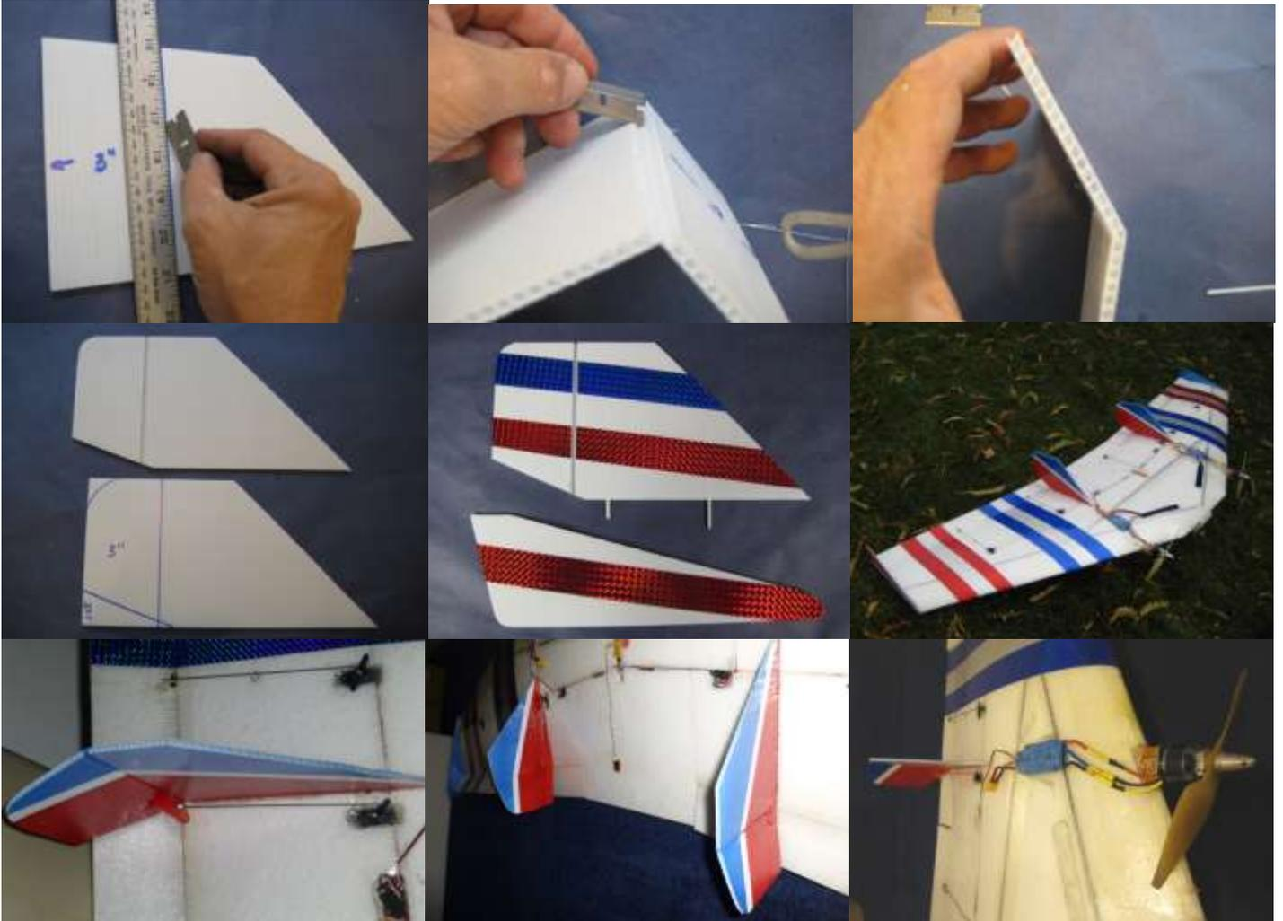
**13. INSTALLING THE TIP FINS The tip fins are part of the landing gear keeping the elevons 1" (2.5 cm) off the ground**
