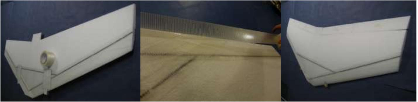
**7. OPTIONAL PAINTING** --- The cores below were painted after the E-taping and before the plane was laminated with Krylon Fusion paint for Plastics. The laminate was applied as soon as the cores could be handled 30 minutes after painting and has stuck well to the EPP foam.
