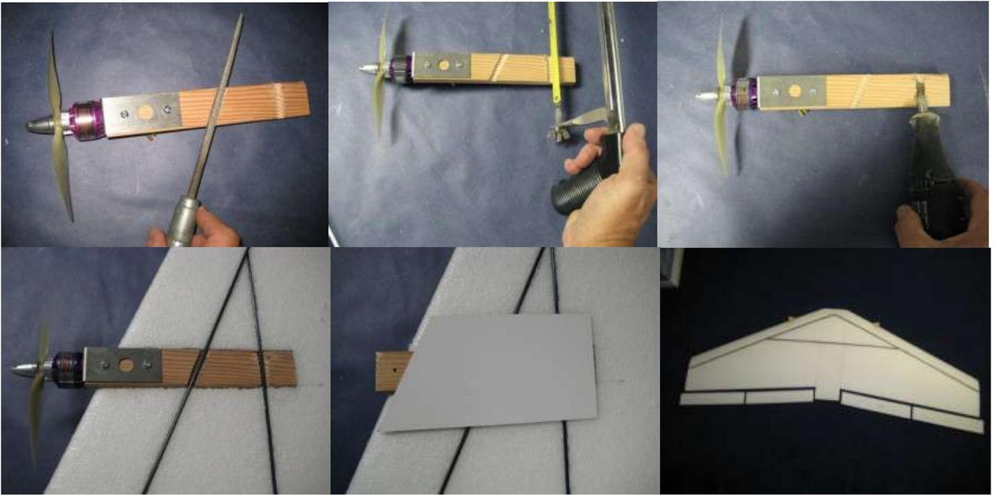
**5. The shock cord keeps the plane from tearing between the elevons in a forward impact**
