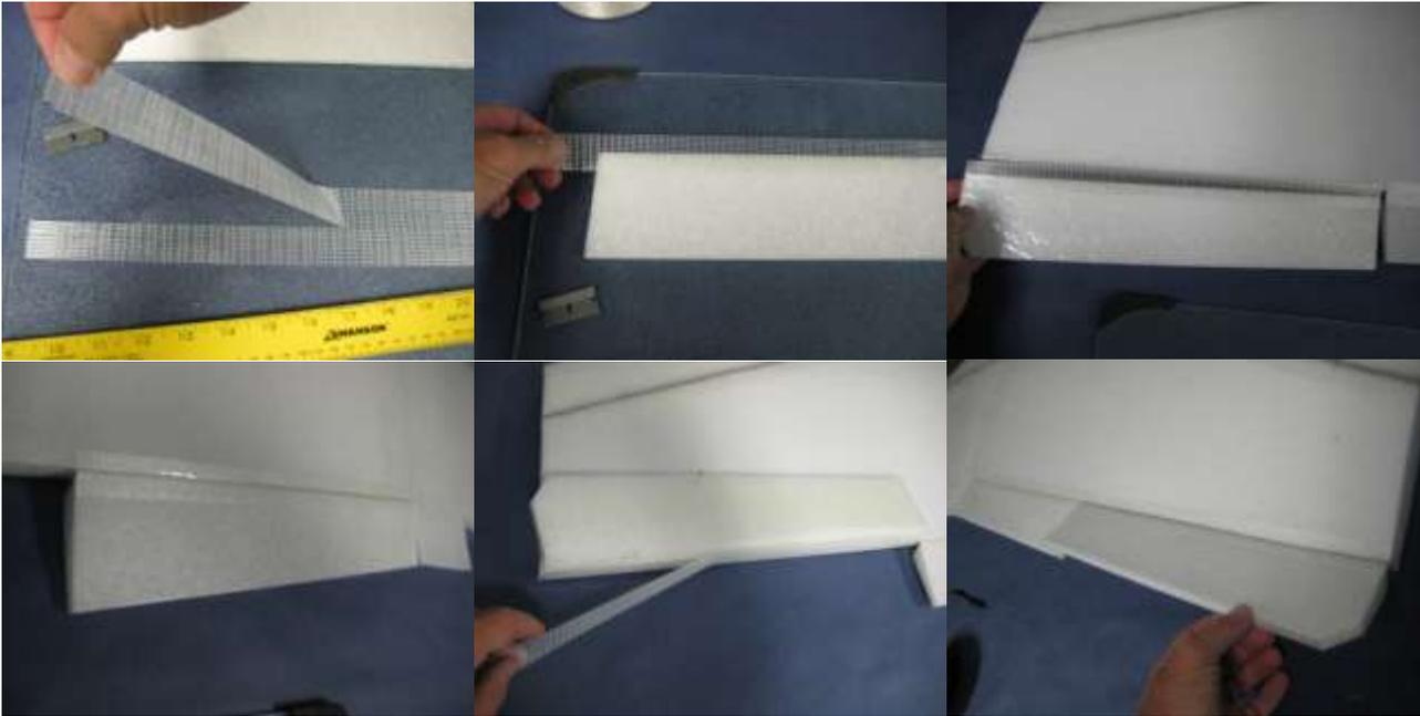
**11. Iron 2" (5 cm) wide laminate strips over tape on both the top and bottom of the hinge line to protect the tape from UV light.**
