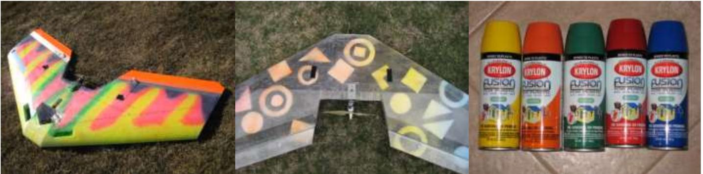
**8. Laminating the wing. You should put a single layer of laminate on top and bottom of wing over foam and tape**
