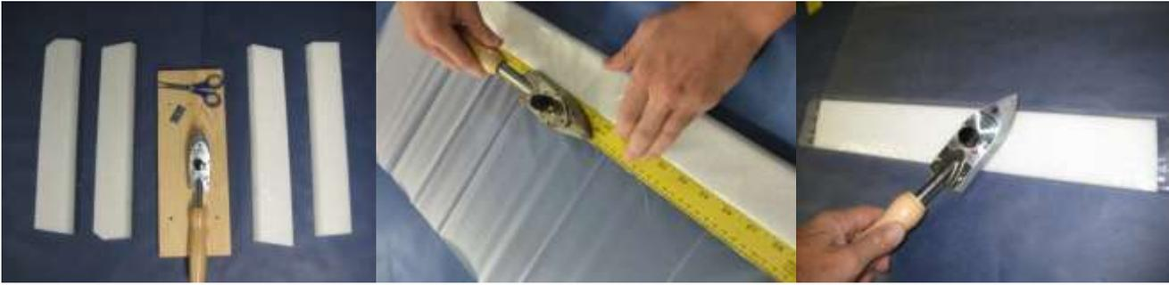
**10. Make a hinge for the elevon with a 1" (2.5 cm) strip of E-Tape on both the top and bottom of the wing.**
