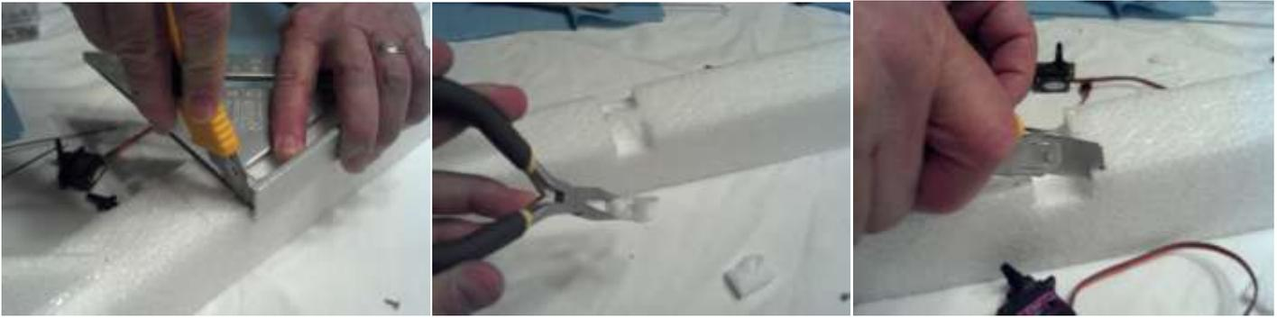
122. Use a straight edge and razor blade to cut across the fuselage at the front and back marks for the servo. Cut only as deep as you need to for the servos to lay flush with the top of the fuselage.
