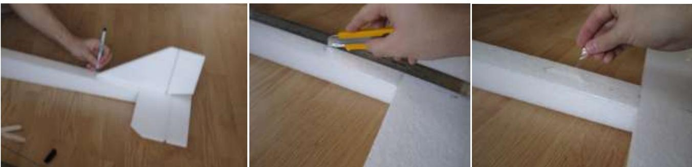
115. Place the rudder on top of the fuselage and horizontal tail piece, so that the back of the rudder lines up with the back of the elevator. Make sure the rudder is centered, front and back, and mark with a pen where the rudder sits on the fuselage.
