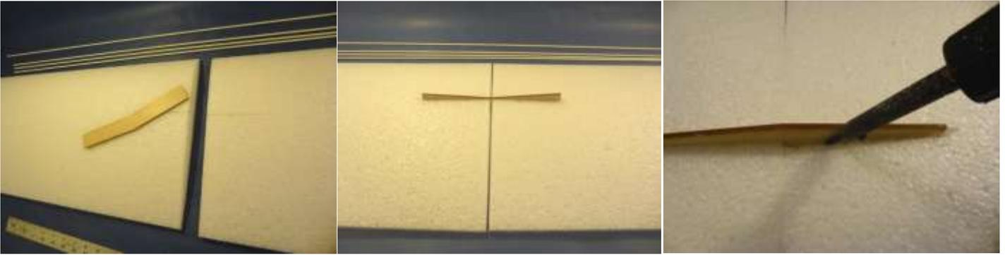
51. Cut the ailerons to length. We like to leave a 1" gap between the aileron and fuselage so there is room to attach the rubber bands.
