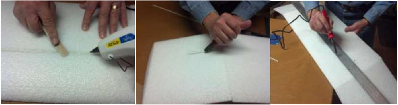
29. Fill in the pre-cut slits in the wing tips with hot glue, especially around the spar that goes through it.
