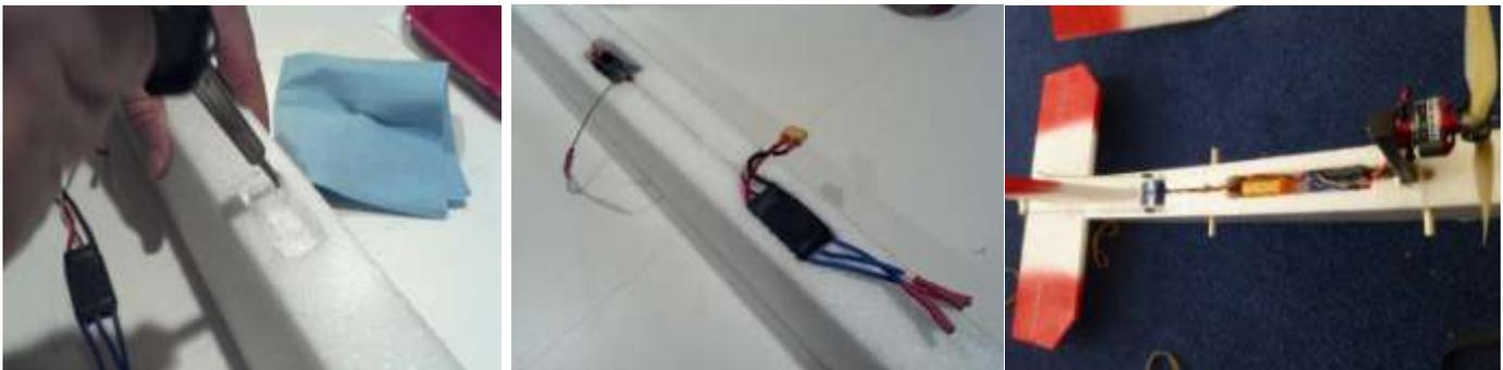
143. Adjust your soldering iron tip to the proper depth, and melt compartments for the ESC and Rx or you can cut them with a longer blade hobby knife. Make the size of the compartments tight so that the ESC or Receiver fit snugly.
