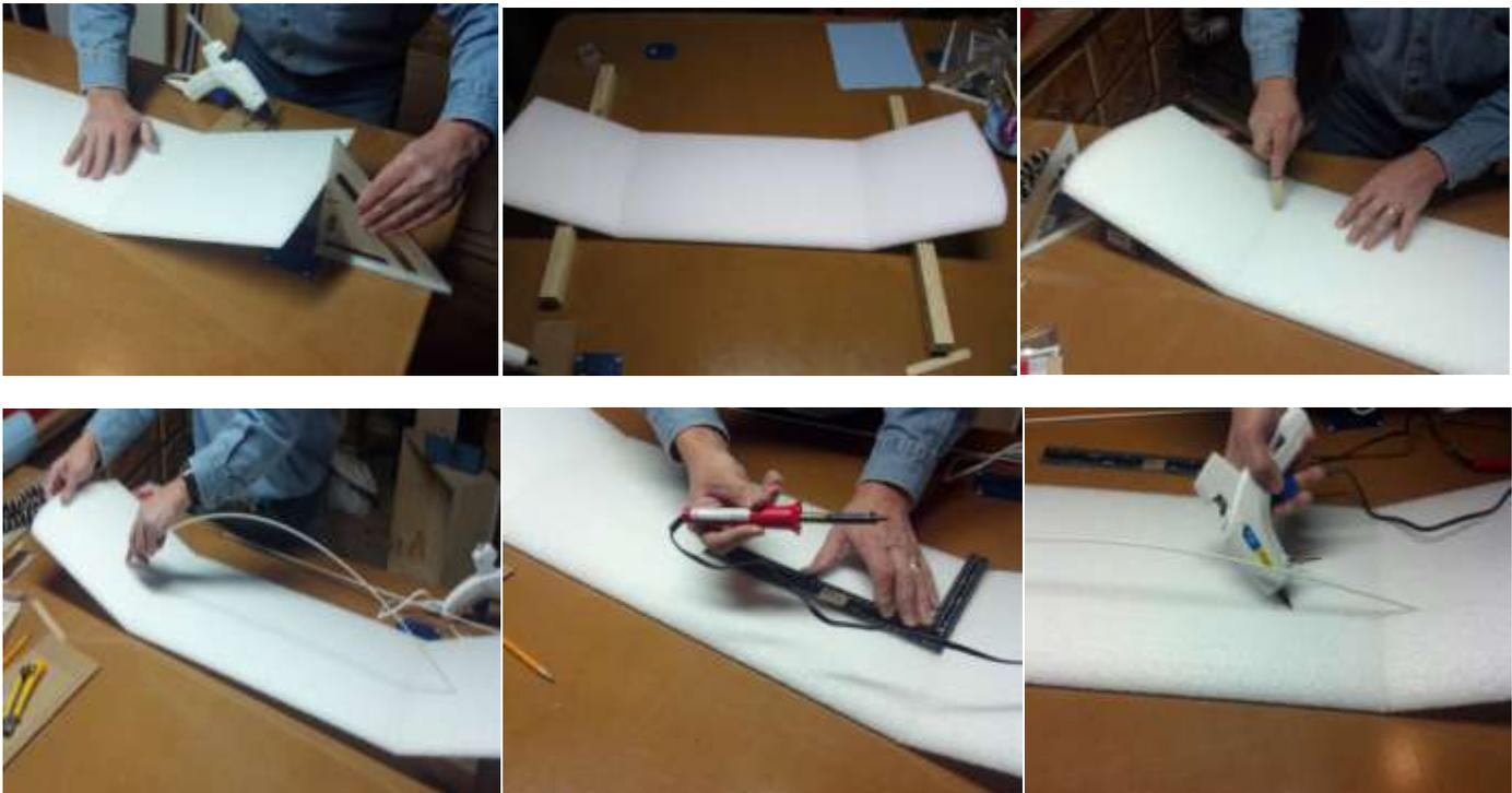
22. Lay the spar on top of the wing, and slide the ends of the spar through the pre-cut slits that are 4" back in the wing tips.
