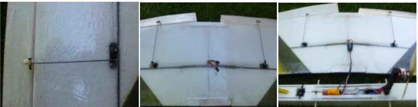
58. Gently push the servo wire into the slit leaving the last 1" of the wire out of the center of the wing.
