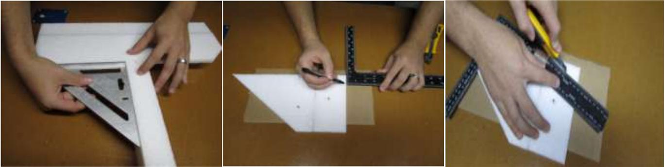
113. On the flap of the rudder (upright tail piece), measure and place a mark 1" (2 cm) up from the bottom.
