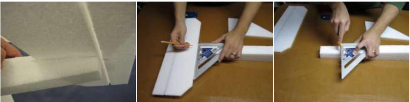
108. Find the pre-cut slit on the top of the fuselage where the horizontal tail and elevator will be attached.
