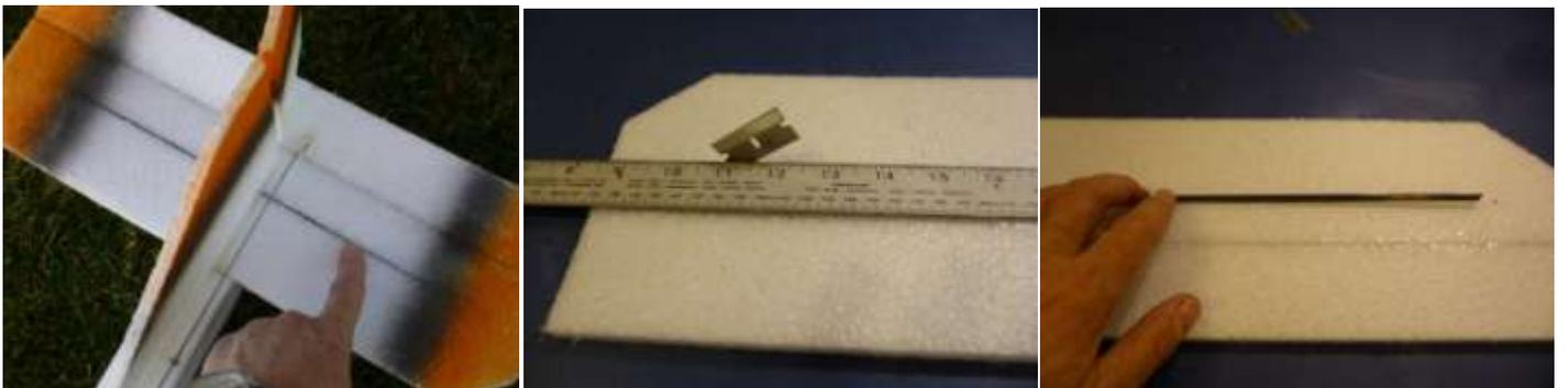
7. You can reinforce the tail with a flat carbon during the build or after the plane is built. The flat carbon spar will be included in all kits in after December 2013. You can easily put a spar in a plane that has already been built.
