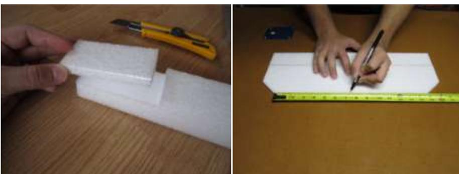
111. Use your ruler to mark the center point at the front and back of the horizontal tail piece. Make a matching center mark on the top of the fuselage, just in front of the piece you just cut out.
