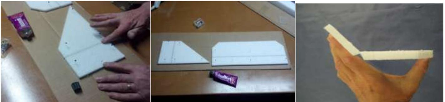
4. Goop is a fast drying glue. Use only in well ventilated areas. The glue will age in the tube once it is opened. Apply it quickly and do not go back to touch it up or it will roll up in little glue balls and can ruin a hinge line.
