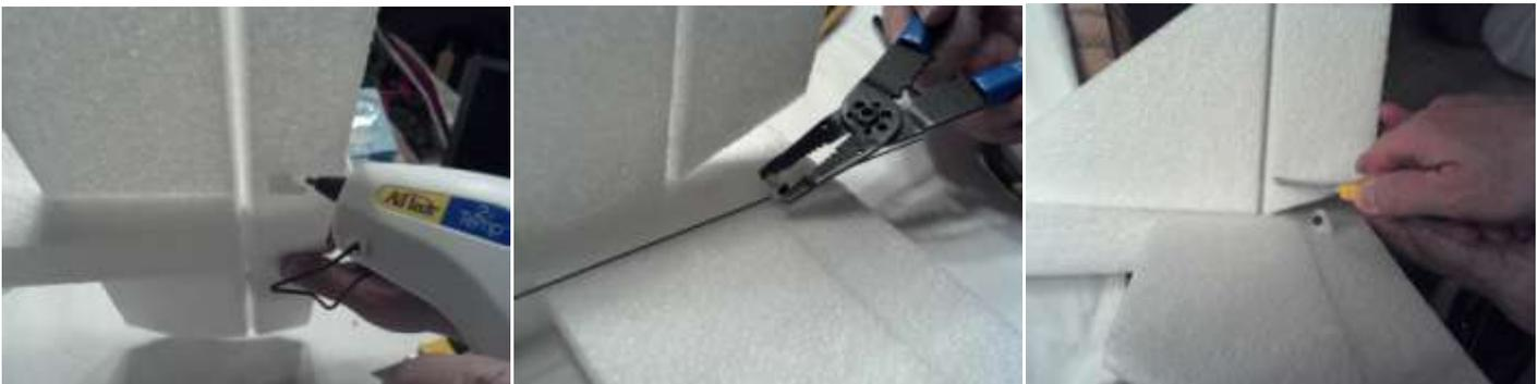
129. Use a pointed blade or box knife to cut a slot completely through the elevator for the horn. Start just behind the hinge line.
