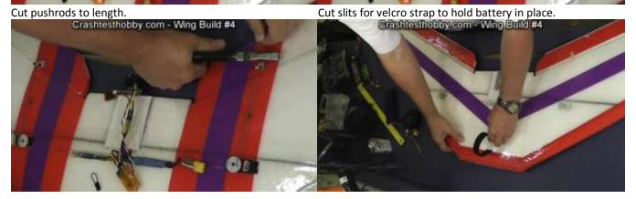
Place battery in place and secure with the Velcro.
