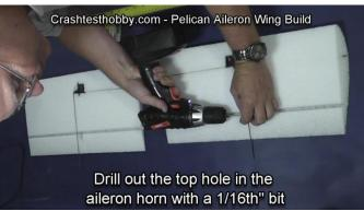
Drill the top hole in the horn with a 1/16" bit. Install the EZ connectors. Trim the push rod to length.
