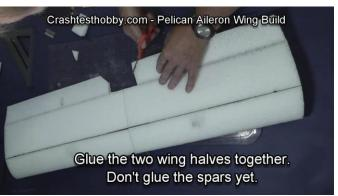
Glue the wing halves together. Apply glue to the center spars after you have the wing positioned with the tip 3.5" off the table. Squeeze liberal amounts of glue in to support the spars where they cross in the middle of the wing.
