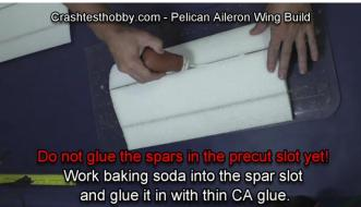
Put baking soda along the spar and work it into the slit with the carbon spar. The baking soda acts as a catalyst and speeds up and hardens the CA glue. Blow off the excess baking soda or it will make hard lumps along the spar. Glue the spar in to the slit with thin CA glue.
