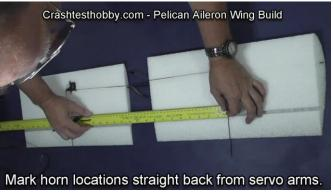
Install the control horn for the aileron straight behind the servo arm poking out the bottom of the wing. The holes for the control horn should be at the hinge line of the aileron. Cut a slit with a hobby knife. Make a small hole along the slit for glue to move up the horn and glue the horn in place from both the top and the bottom.
