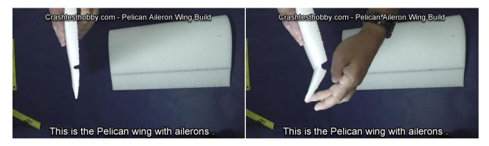
The ailerons are already precut into the wing core. Fold up the ailerons and flex the wing to loosen up the hinges.
