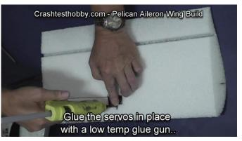
Cut a slit in the wing deep enough to hide the servo wires. Before gluing the servos in place with a low temperature glue gun, bind them to the radio and center the servo arms on the servo. Drill out the third hole in the servo with a 1/16" bit to be big enough for the push rod. Don't glue the servo extension wires in except for where they exit the wing in the middle where they will be plugged into a Y connector that plugs in the receiver.
