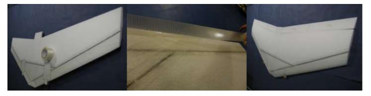
7. OPTIONAL PAINTING --- The cores below were painted after the E-taping and before the plane was laminated with Krylon Fusion paint for Plastics. The laminate was applied as soon as the cores could be handled 30 minutes after painting and has stuck well to the EPP foam.
