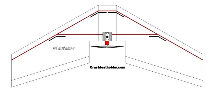
**The spar location on the top and bottom Gladiator are the same.** The fiberglass spars are installed directly over each other to create and "I beam" type structure that is many times stiffer than one spar alone.
