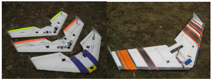
We recommend that you build and laminate the plane before you install the radio. This makes the plane easier to build and easier to service and repair It saves time when you need to trade out electronics giving the plane a longer life with less work. You will notice in the pictures that some flyers use the extension and some do not. One of my favorite builds left out the extension and put the motor on the nose.
